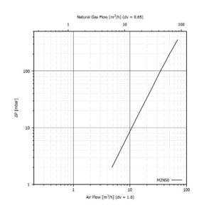
P burner = 3 mbar Flange = Rp3/4"
