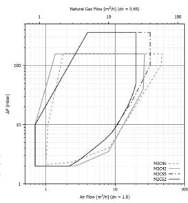
P burner = 3 mbar Flange = Rp3/4" Maximum flow can be reduced when other flanges are connected with.
