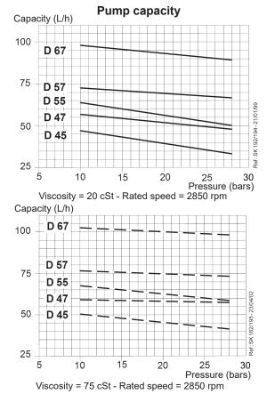
Data shown take into account a wear margin. Do not oversize the pump when selecting the gear
